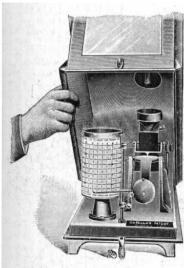
FIG. 1.—New Casella recording rain-gauge.
