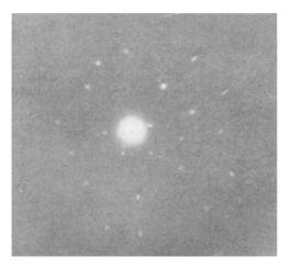
obtained on transmission through an antimony crystal are shown in the adjoining photograph. Owing, however, to the difficulty of procuring individual crystals of the metals, symmetrical Laue patterns have not yet been obtained. The experiments, however, show that this method of investigating metallic crystals may prove very helpful to the metallurgist.
