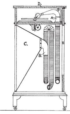
out through the trumpet was so considerable that it made very little difference whether the lid was closed or open; with the new arrangement this scraping is eliminated to so great an extent that until the felt was inserted quite an appreciable amount of noise was found to come out round the lid.
