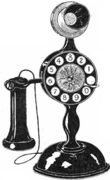
FIG. 1.—Subscriber's Telephone, with calling arrangement.
