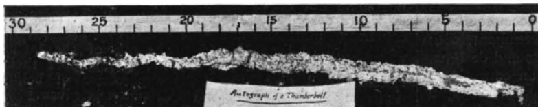
Photograph of the cast of a hole formed in ground by a lightning discharge.
