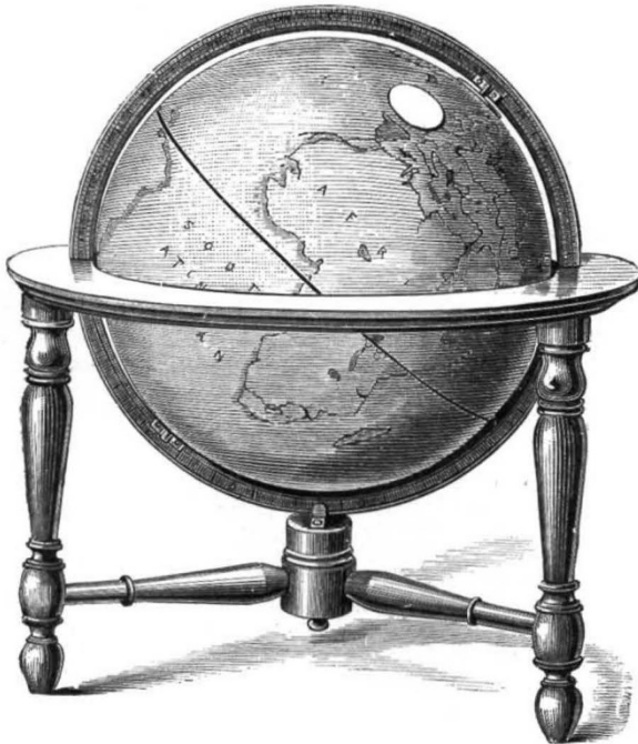
FIG. 6.—In this case the axis is inclined to the wooden horizon, which is parallel to the horizon of Britain when at the top of the globe. The wafer representing the horizon of Stonehenge is carried obliquely up and down in a direction parallel to the equator, so that the sun and stars rise obliquely to the horizon.
