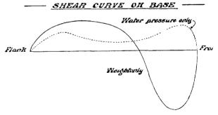
ments at University College showed that this base shear due to the weight of the dam only was as important as, and probably more important than, the distribution of shear due to the water pressure.
