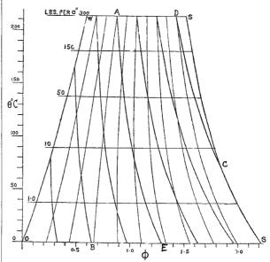
the place of throttling is well protected from loss of heat by a non-conducting covering, and in this case total heat remains constant. Now if the line DC is looked at, it will be seen that steam which is 90 per cent. dry at 300 lb. pressure, if throttled to 150 lb. pressure is about 93 per cent. dry, and if throttled to 50 lb. pressure is about  $95\frac{1}{2}$  per cent. dry. Thus the drying effect is not very great.
