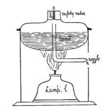
the small subsidiary lamp I. be removed from the position shown in the sketch and then placed from three to four inches in front of the nozzle, a blue flame cone will in a second or two dart back from the flame of L to N. The lamp L may now be completely removed, and the flame cone will continue—adder tongue like—to dart back and forth between N and a point three to four inches distant for hours together.
