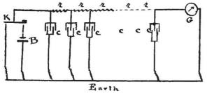
earth, rrare a number of high resistances which play the part of the conducting core of the cable, and c c are the capacities which play the part of the insulating sheath of the cable. G is the galvanometer, one side of which is connected to earth, and forms the
