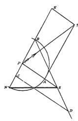
duced, so that PA = PB = PN. Take C in BN, so that BC measured towards N equals PS. Draw CD parallel to PS, D being in the line BS. Measure PE away from N, so that PE = CD. The diagonal PT of the parallelogram AE is the
