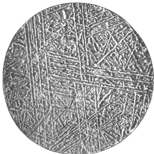
FIG. 1.—Silver-lead eutectic, \times 100 . Oblique illumination.
