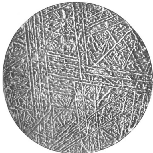
FIG. 1.—Silver-lead eutectic, \times 100 . Oblique illumination.
