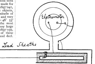
wire from inductive effects, it was surrounded by a tube of lea connected to sheaths.
