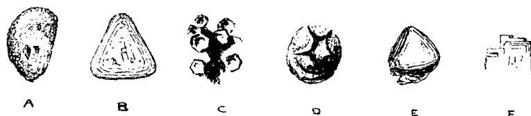
FIG. 8.—Preparations for the microscope of diamonds and other forms of carbon obtained from carburised iron.
