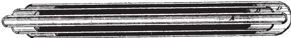
FIG. 5.—Longitudinal section of the Ferranti main. A, inner copper tube; B, outer copper tube; D, iron protecting tube; waxed paper insulation shaded black.
