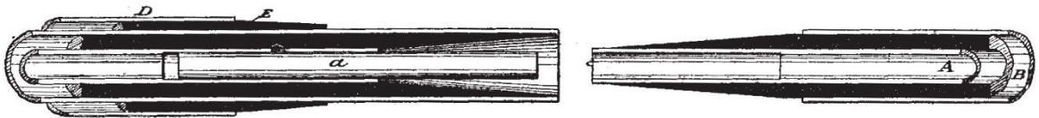
FIG. 7.—Ends of two pieces of main, tapered ready for jointing. a , copper rod to make electric connection between inner copper tubes; e , waxed paper coned like a pencil.
