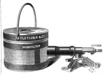
heat, nor will they hold their shape at any temperature ap proaching whiteness. The burner alone will be useful in heating many substances in the open, but, owing to the broad and diffused flame, it is of little practical value for blow-pipe work.
