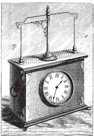
the principle of torsion. It has to be wound up daily, and the phase of the pendulum—that is to say, the time which elapses between two identical positions of the regulating system—is six seconds. The general mechanism does not differ from that of ordinary clocks; we find the main spring and other usual parts, and a train of wheels giving rotation to a vertical axis which is seen over the case and the rate of motion of which is to be regulated.
