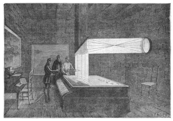
face of the water, no sign of their presence being apparent. A metallic wire connects each of them with a post of observation situated on the coast at a point sufficiently elevated to permit of the port being seen. According to well-known optical laws, an image of the port is formed on the glass. Black points marked on that image indi-
