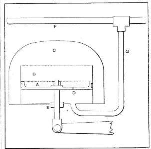
power, the vacuum being created by means of an ejector on the engine, connected to every vehicle on the train by means of a continuous pipe, having flexible pipes and couplings between the vehicles. To maintain the vacuum throughout the train against leakage, there is a small ejector continually in use on the engine.
