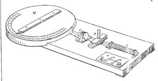
was placed end-on to the needle, and its directive action was diminished at will, not by turning it round on its centre, but by shifting it to a greater distance along a linear scale below it. The form now given by Hughes to linear scale below it. The form now given by Hughes to the balance is one of so great compactness and convenience that it will probably prove a most acceptable addition to the resources of the physical laboratory.
