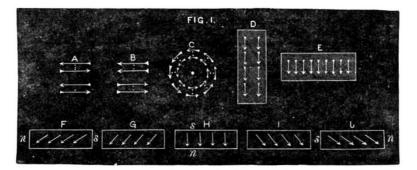
neutrality consists of a closed chain, or circle, as by torsion we can partially deflect them on either side; thus, from a perfect externally neutral wire, producing either polarity, by simple mechanical angular displacement of the molecules, as by rightor left-handed torsion.
