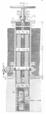
easily replaced. On the other hand, the unsuitable nature of the towing line for transmitting torsional force, is obvious. Further, the slip of the fan must by seriously affected by the constant variation, in length, of the submerged portion of the line. In Walker's log these difficulties are partly met by the use of a governor, consisting of a pair of weights fixed to the towing line, and revolving with it; but this device can only modify the evil.
