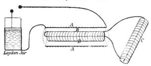
(2) Now arrange the coils as shown, A as primary, B as secondary, C in the circuit of B, and a needle in C. Let there be no break in the circuit of B and C.
