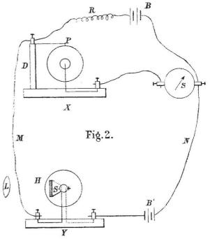
the sensitised paper and the selenium exposed to a strong light, the resistance R was varied until the galvanometer needle came to rest at zero. If the two batteries were similar this would occur when the resistance of R was made about equal to that of the selenium cell in the light. The point now made no mark when drawn over the paper. The selenium cell was then darkened, and the point immediately traced a strong brown line; a feeble light was next thrown upon the selenium, and the intensity of
