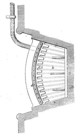
tity of ashes that will be produced by combustion of the coke and anthracite in the front part of the grate discharge themselves down the incline towards the back of the hearth, where an open ash-pan may be placed for their reception.
