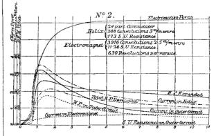
An observation in Sir Charles Wheatstone's paper is referred to, pointing to the fact that a powerful current is set up in the shunt circuit of a dynamo-electric machine, which circumstance has since been taken advantage of to some extent by Mr. Ladd and Mr. Brush, in constructing current generators.
