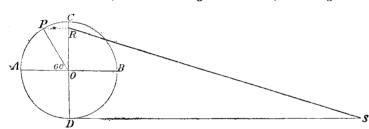
draw PR at a right angle to DC. Connecting the points S and R you will find the length RS very nearly equal to the circumference of the circle.
