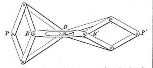
at o; and the poles R and R' are connected together by a bar with a slot in it, through which the pin which forms the pivot at o passes. Then if P, R, P', R, are constrained to keep in a straight line, P and P' can approach or recede from 0, only in such a way that, if there is a lens of proper focal length at 0, P and P' will always be conjugate foci.
