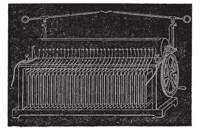
The tension of a secondary battery of 800 couples is not necessary to produce marked effects with this apparatus. By putting in action only 200 couples, we have sparks of eight millimetres, and we may, without doubt, by diminishing still more the thickness of the insulating plates and multiplying the number of condensers, obtain effects with a source of electricity of less tension.
