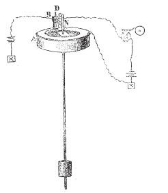
falls, breaks contact with p and makes contact with C, which thus tends to pull the needle over to C, and so on; in this way the pendulum receives at each oscillation the impulse necessary to overcome the forces tending to stop it; and thus will keep oscillating as long as the battery supplies the motive power. For small arcs the beat is not affected by variation in bettery power.
