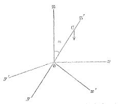
perpendicular to 0x'. Let  $w' = weight of wheel and axis; <math>\mathcal{A}, \mathcal{B}, \mathcal{B}$ , moments of inertia round 0z, 0x', 0y';  $w_2$  angular velocity round 0y' at time t; a =the distance of C. G. from 0z, 0z' $x_0x' = \phi$  = angle described by ox' in time t. Taking moments about 0y', we have
