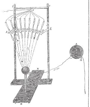
apparatus of M. De la Rive, who placed his current in vacuo, and did not show the property of ordinary atmospheric air of allowing to pass unobserved at the pressure of 760 mm. a stream of electricity which illuminates a rarified atmosphere. The experiment is most attractive, and hundreds of persons witness it every day.
