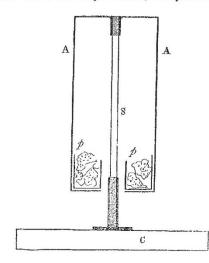
left till morning. The experiment was then performed thus The gold leaves of the electroscope were connected with A A by a fine wire and a charge communicated; the gold leaves at first repelled each other, but almost immediately collapsed. This was repeated once or twice, to show distinctly that there was no insulation.
