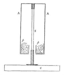
left till morning. The experiment was then performed thus The gold leaves of the electroscope were connected with AA by a fine wire and a charge communicated; the gold leaves at first repelled each other, but almost immediately collapsed. This was repeated once or twice, to show distinctly that there was no insulation.
