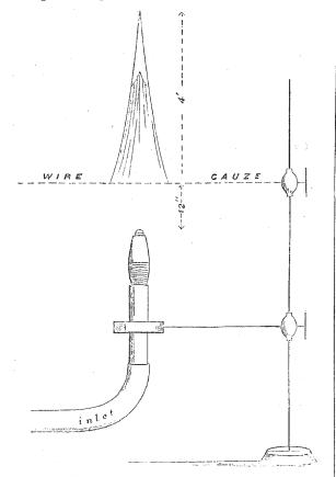
inches square, resting on the ring of the retort-stand ordinary window-blind wire-gauze 32 meshes to the lineal inch. The burner was Sugg's steatite pin-hole burner, the same as used for vowel flame.
