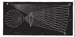
woodcut, from the recent work of Dr. Williams of Boston, where the rays of light emanating from the star are reflected from the concave mirror DE, and rendered convergent by the lens L, lighting up the whole of the posterior surface of the globe; some of the rays returning from this pass through the opening in the mirror, and are seen by the observer at O. The precise mode in which the image is formed is shown in the following cut, borrowed
