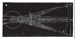
from the same work. The rays returning from N, N' N" representing a portion of illuminated fundus, are brought to a focus by the convex lens L, at A, A' A", and then form,
