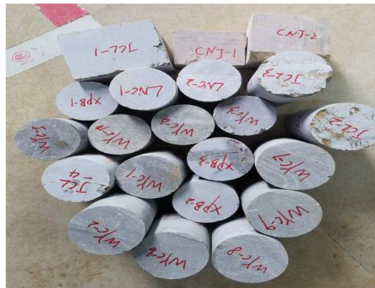
Figure 6. Processed partially Sandy Dolomite core sample.
