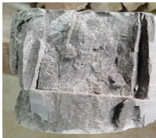
Figure 7. Rock core after UCS test.
