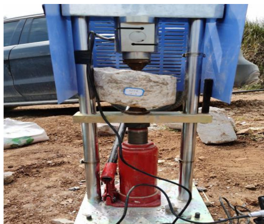
Figure 9. Field tests of PLT.
