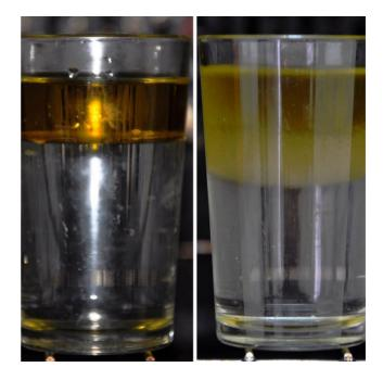
Oil-water illustration of spin-gradient thermometry At low temperatures, oil and water do not mix and form clearly separated phases with a tiny interface (left). At higher temperatures, the interface region is considerably larger, allowing one to deduce the temperature of the fluids (right).
