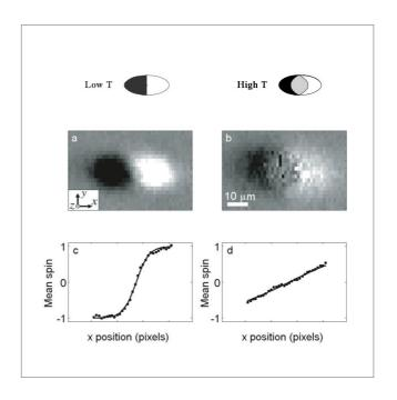
Spin-gradient thermometry experiment with Mott insulators At low temperatures, the two components of the quantum gas — *spin up* and *spin down* — are clearly separated (a), whereas they overlap considerably at higher temperatures (b). Image analysis (c,d) allows one to deduce the temperature by comparison to the known, theoretical temperature dependency of the two phases and their interface region.
