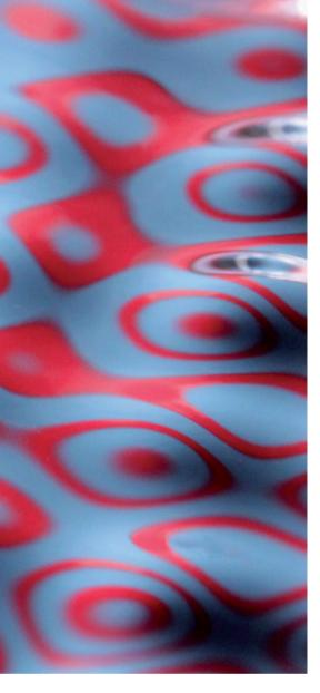
An experiment showing that oil droplets can be propelled across a fluid bath by the waves they generate has prompted physicists to reconsider the idea that something similar allows particles to behave like waves.
