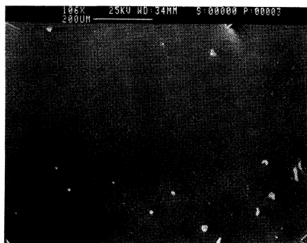
Figure 9. SEM micrograph of the fracture surface of a PDMS-modified \text{SiO}_2 glasses having low PDMS content, at a magnification of 106\times .
