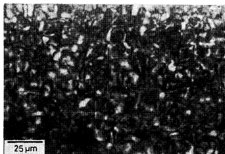
Figure 4. Polarized optical micrograph of an EC/PAA composite prepared from a 50 wt% EC/AA solution by polymerizing AA.
