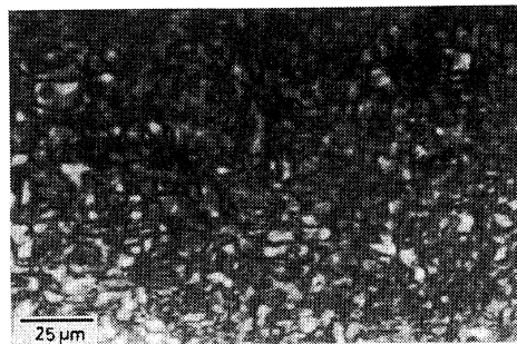
Figure 2. Polarized optical micrograph of a 55 wt% EC/AA solution.
