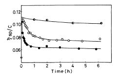
Figure 1. The viscosity change of a chitin solution of methanesulfonic acid at  $0^{\circ}$ C ( $\bigcirc$ ),  $25^{\circ}$ C ( $\bigcirc$ ), and  $40^{\circ}$ C ( $\bigcirc$ ).
