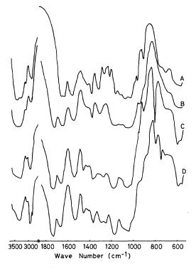
Figure 2. Infrared absorption spectra of chitin and acylchitins: A, chitin; B, 1.4 formylchitin; C, 1.9 propionylchitin; D, 1.8 butyrylchitin.
