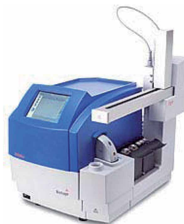
Figure 2 | Initiator eight single-mode microwave reactor from Biotage AB (Uppsala).
