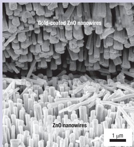
opposing sets of nanowires allow only negative charge to pass from the bare nanowires to the gold-coated nanowires. This, in turn, generates a voltage across the two strands.
