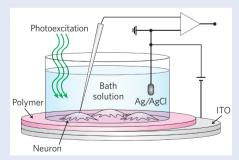
polymeric light-sensitive film made from rr-P3HT:PCMB, a fullerene–polythiophene blend commonly used in organic solar cells. The researchers cover one side of the film with indium tin oxide (ITO) to form a transparent electrode, and the other with neurons surrounded by an aqueous salt solution, which keeps them alive for up to 28 days.
