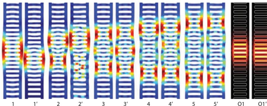
Photonic crystals are periodic structures that guide and trap light, whereas phononic crystals do the same for mechanical vibrations or sound. Oskar Painter and colleagues at the California Institute of Technology have now created optomechanical crystals that can act as both photonic and phononic crystals (*Nature* **462**,
