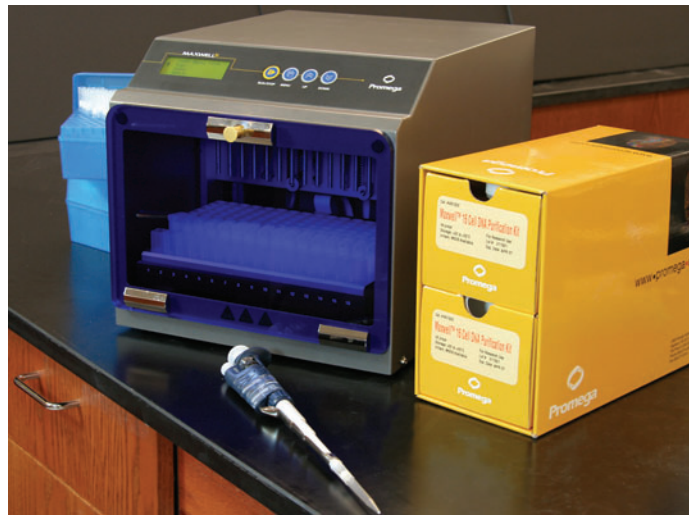
The Maxwell 16 System from Promega offers benchtop automation of nucleic-acid purification. (Courtesy of Promega.)
