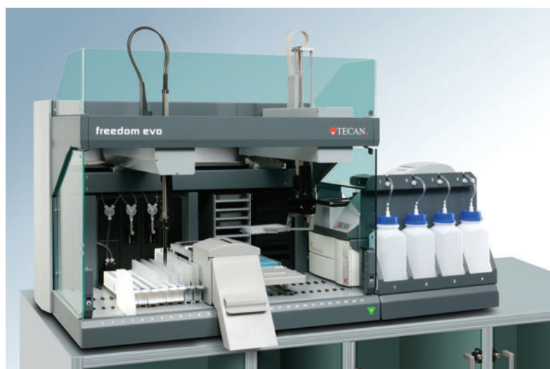
The Freedom EVO 75 represents the smallest and most economical of Tecan’s versatile platforms for lab automation. (Courtesy of Tecan.)
