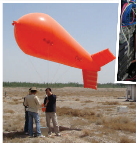
Clockwise, a balloon used to measure dust; collaboration participants; and a collection of radiometers.
