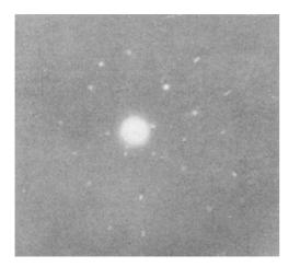
obtained on transmission through an antimony crystal are shown in the adjoining photograph. Owing, however, to the difficulty of procuring individual crystals of the metals, symmetrical Laue patterns have not yet been obtained. The experiments, however, show that this method of investigating metallic crystals may prove very helpful to the metallurgist. E. A. OWEN.
